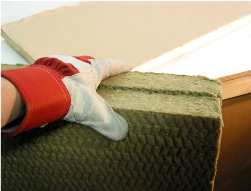
4" of 8 lbs. pcf density Rockwool: less rigid than 703, much heavier, tends to be flakey, inexpensive, excellent acoustic properties.
