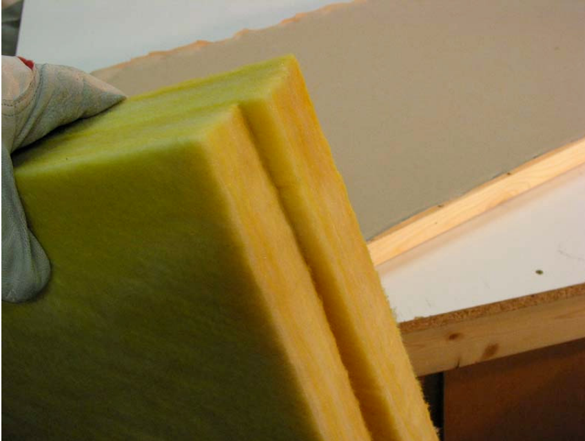
4" of 3 lbs. pcf density semi-rigid fiberglass board [703]: light weight, rigid, durable, excellent acoustic properties.
